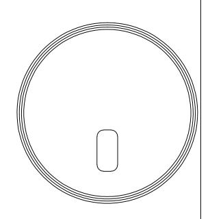
CAST IRON TO CONFORM TO ASTM A-48, CLASS 30B A - 1024
